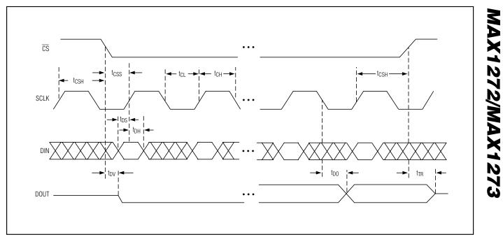
Figure 4. Detailed Serial Interface Timing
