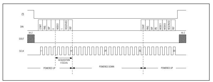
Figure 9. Immediate Power-Down Timing
