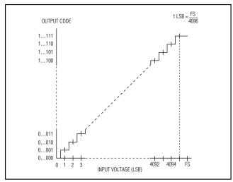
Figure 13a. Unipolar Transfer Function
