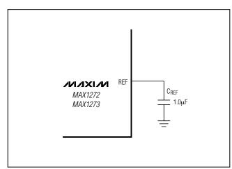
Figure 7a. Internal Reference Configuration
