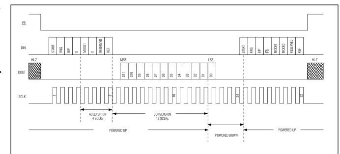
Figure 8. Delayed Power-Down Timing
