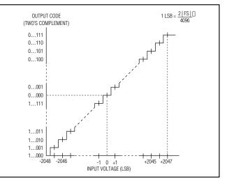
Figure 13b. Bipolar Transfer Function
