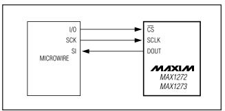
Figure 10b. MICROWIRE Connections
