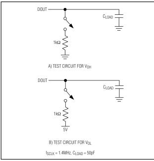
Figure 1. Output Load Circuit for Timing Characteristics
