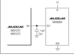
Figure 7b. External Reference Configuration
