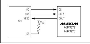
Figure 10a. SPI Connections
