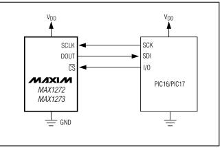
Figure 12. SPI Interface Connection for a PIC16/PIC17
