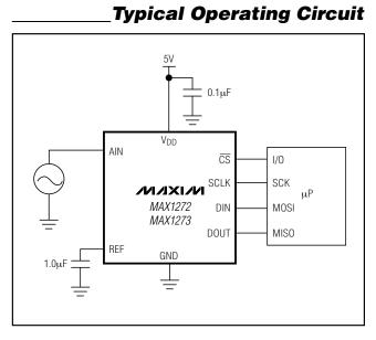
Figure 14. Power-Supply Grounding Connections
