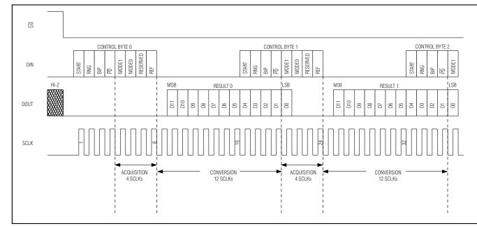
Figure 6. Conversion Timing, 16 Clocks/Conversion
