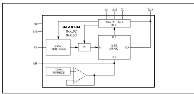
Figure 2. Simplified Block Diagram
