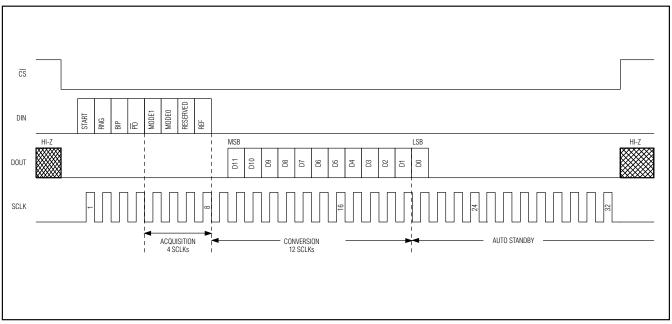
Figure 5. Conversion Timing, 21 Clocks/Conversion
